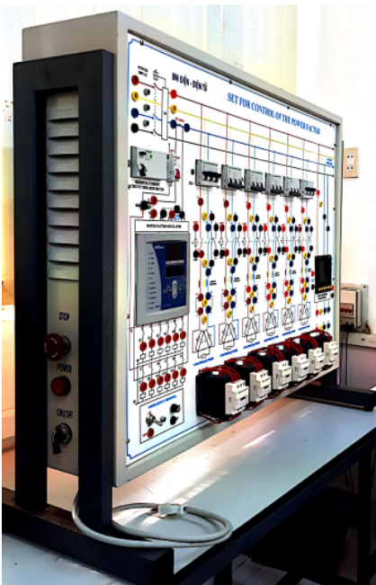
Fig. 1: Reactive power compensation model uses Mikro PFR120 relay
