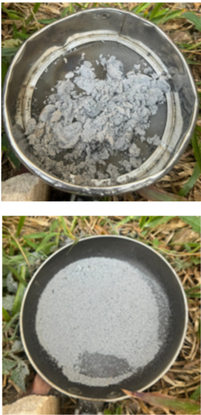
Fig. 6: The biochar from the SCB after the slow pyrolysis process
