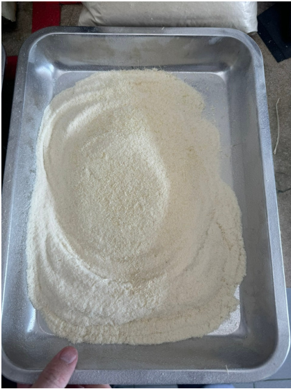
Fig. 4: The SCB powder after drying, blending, and sifting
