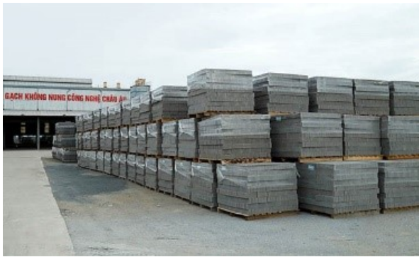
Fig. 5: Fly ash in unburnt brick production [9]
